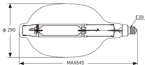
適合安定器 Matching Ballast 匹配镇流器 **KE34P, KD30CP, KD32P, KD30EP, KD32EP, KT32PHV (50Hz), KT41PHV (50Hz)**
