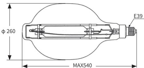
適合安定器 Matching Ballast 匹配镇流器 **KD30CP, KD32P, KD30HP, KD32HP, KD32PHV (50Hz)**
